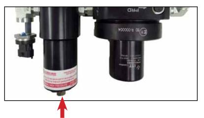
NOTE: For the 2018 model year, the bleeder valve plug is located on the coalescing filter.
