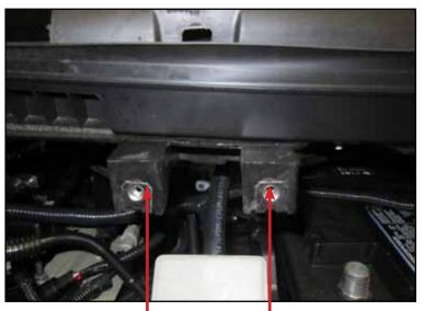
Remove these two tabs. Make a clean cut and flush with the plastic panel. Note: Picture displayed is for driver side, this must ONLY be done for the passenger side. **Do not touch the driver side tabs.**
